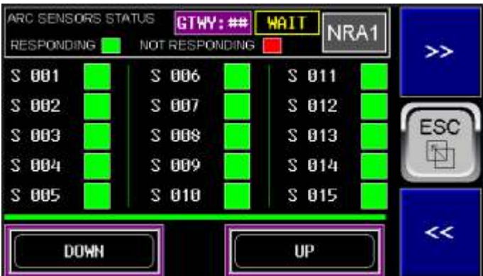
NOT RESPONDING NRA1 to NRA7: (Mono and Multi Gateway) Accessed by pressing <ARC SENSOR NOT RESPONDING>
